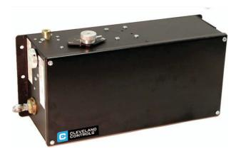
Used in single boiler positioning systems, the MASTER REGULATOR is its own complete, self-contained system for positioning fuel or air or both, maintaining a selectable pressure or temperature control set point. Remote position indication and automatic or manual operation is available.
