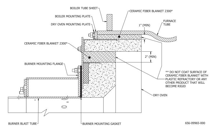
FIGURE 2-1. Dry Oven Installation
