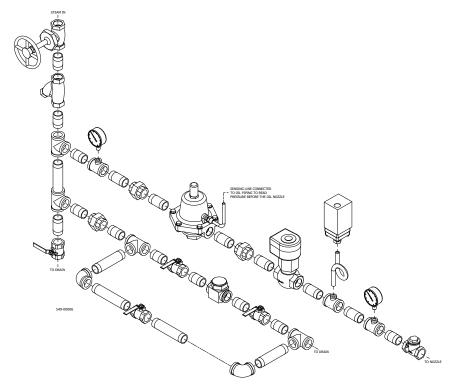
FIGURE 7-3. Atomizing Steam/Top Loaded with Oil
