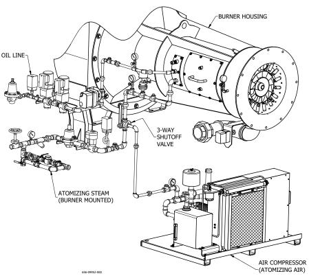
FIGURE 7-1. Steam Atomizing System
