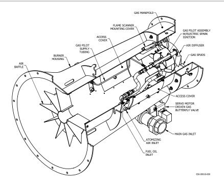
FIGURE 1-1. Burner Housing
