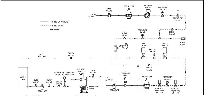
FIGURE 2-2. No. 2 Oil Loop / Atomizing Air Piping Arrangement
