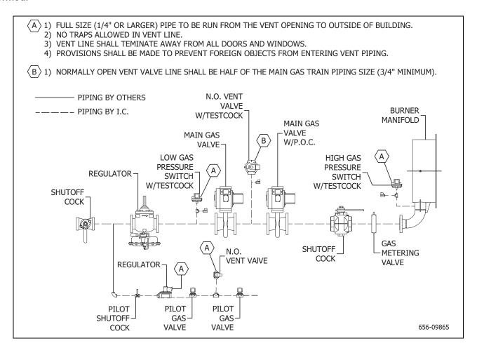
FIGURE 2-3. Gas Piping Arrangement
