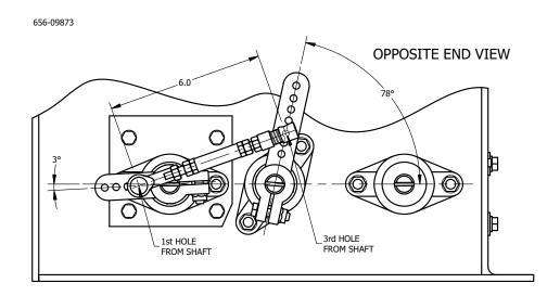
FIGURE 4-1. Firing Rate Control Positions
