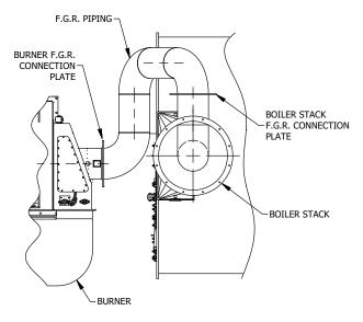
FIGURE 8-2. FGR Connection to Boiler Top View
