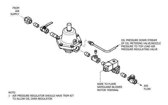
FIGURE 7-4. Plant Air System/Top Loaded with Oil
