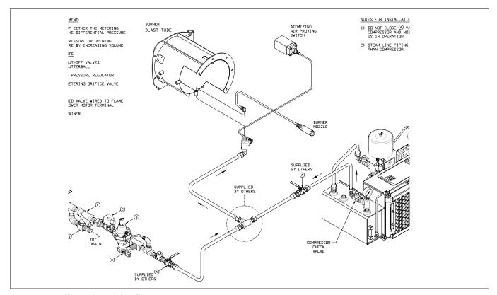
FIGURE 7-1. Steam Atomizing System
