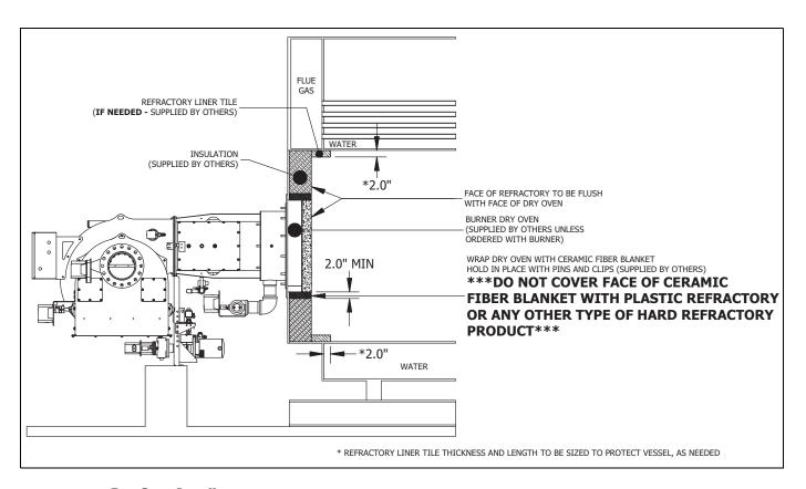
FIGURE 2-4. Dry Oven Install
