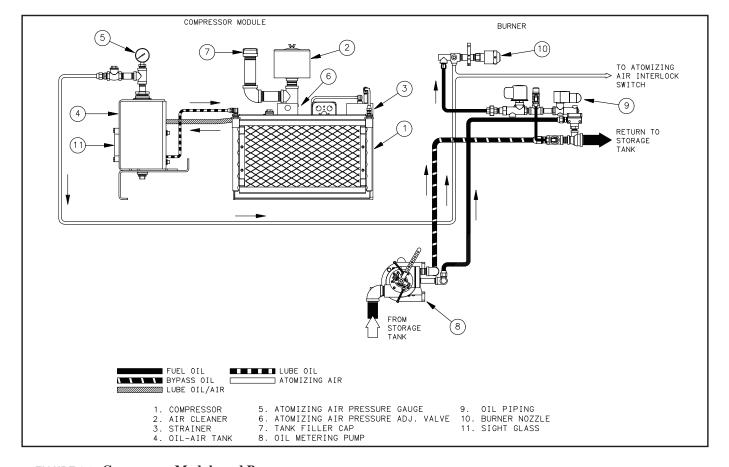
FIGURE 1-3. Compressor Module and Burner
