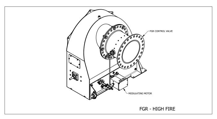
FIGURE 8-3. FGR Control Valve and Control Positions
