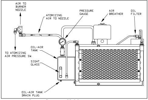
FIGURE 2-5. Separate Compressor Module
