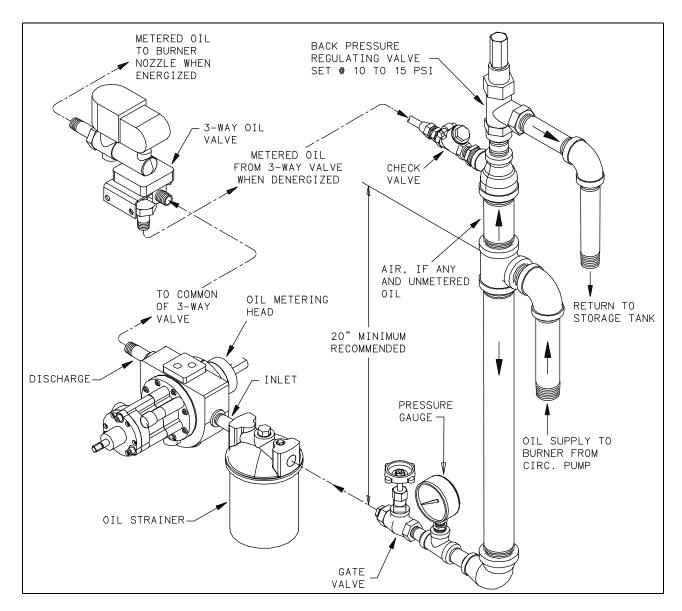
FIGURE 2-6. Typical Oil Supply Loop
