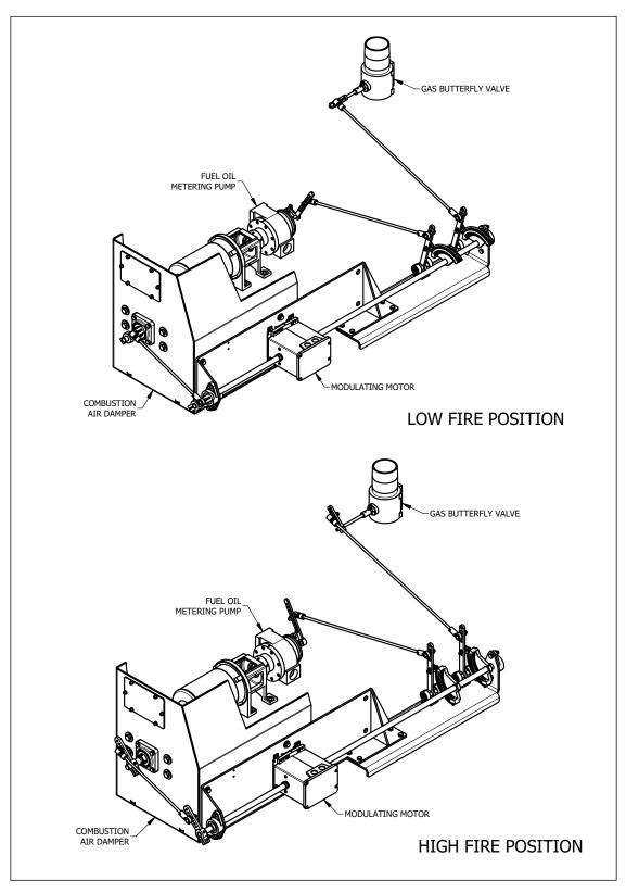
FIGURE 4-2. Firing Rate Control Positions
