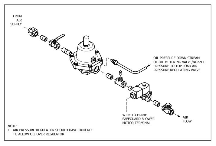
FIGURE 7-4. Plant Air System/Top Loaded with Oil
