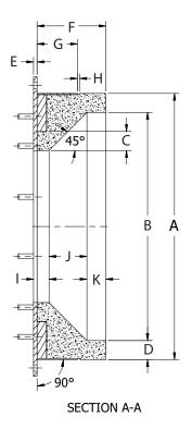
FIGURE 2-3. E-Series Refractory Dimensions
