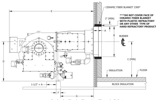
FIGURE 2-1. Combustion Chamber Dimensions (Watertube Boiler)
