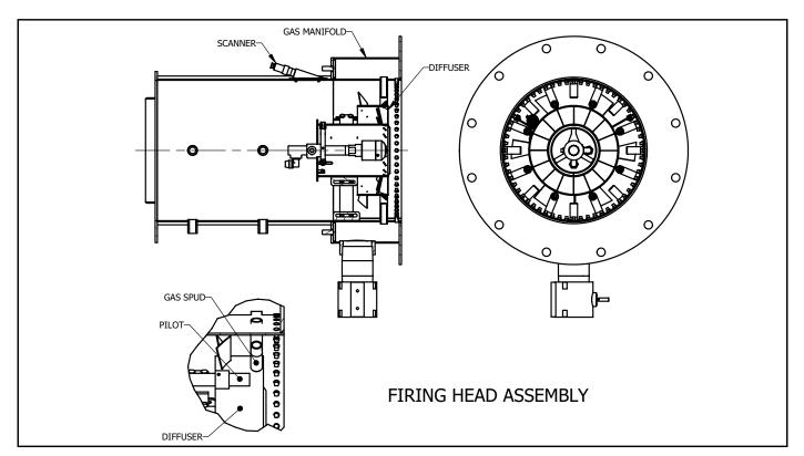
FIGURE 5-1. Firing Head Assembly
