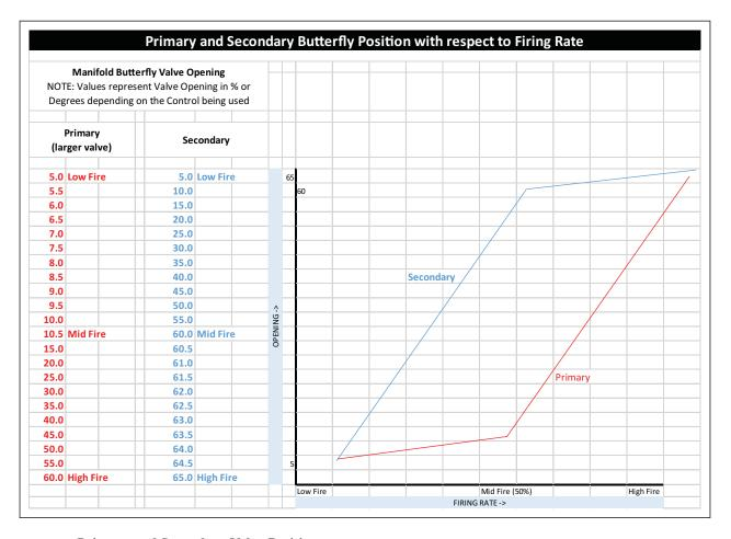
FIGURE 4-4. Primary and Secondary Valve Positions
