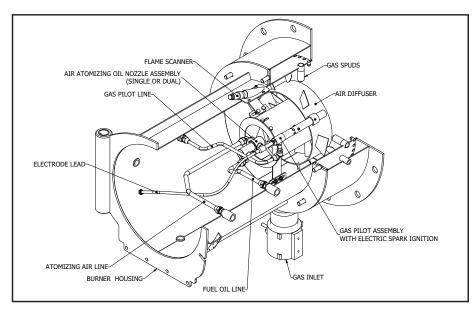
FIGURE 1-1. Burner Housing
