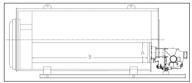
FIGURE 2-2. Combustion Chamber Dimensions (Firetube Boiler)
