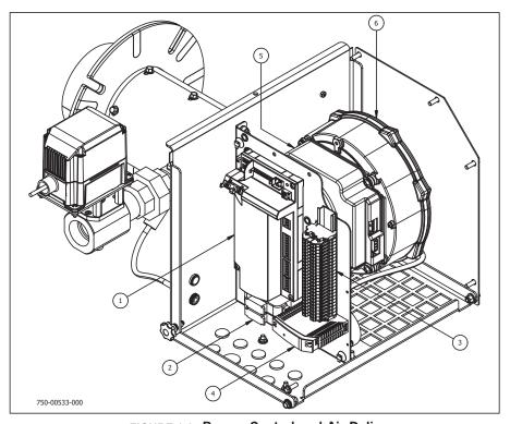
FIGURE 1-2. Burner Control and Air Delivery
