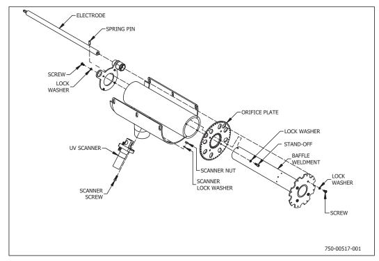
FIGURE 1-5. Burner Housing, Exploded View
