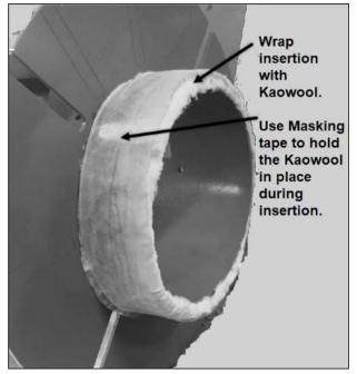
FIGURE 2-4. Insulate Insertion
