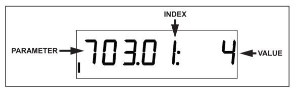
FIGURE 6-1. LMV3 Fault History Example with Indexes
