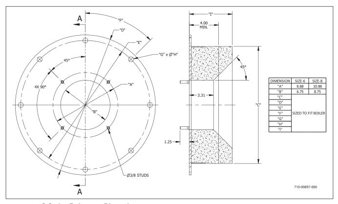
FIGURE 2-3. Q Series Refractory Dimensions
