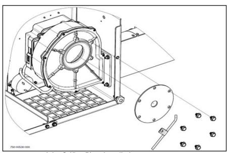
FIGURE 2-8. Inlet Orifice Plate Installation
