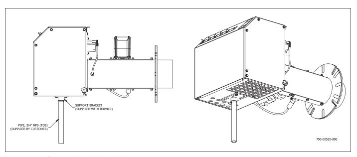
FIGURE 2-6. Support Bracket Installation
