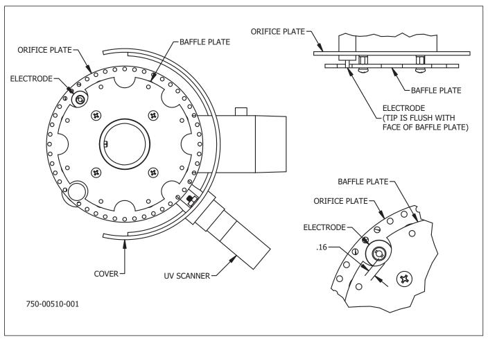
FIGURE 5-1. Ignition Electrode Gap
