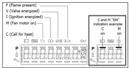
FIGURE 3-1. AZL Status Indications for Normal Operation
