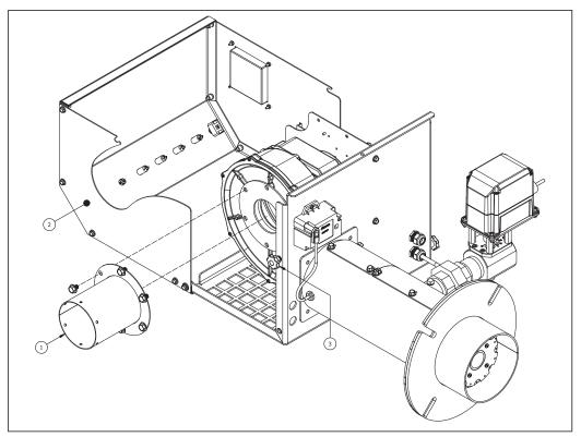
FIGURE 2-7. Ducted Combustion Air
