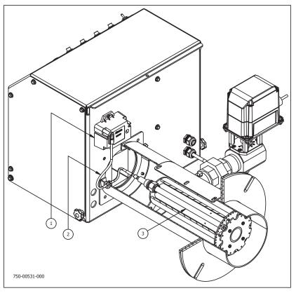
FIGURE 1-3. Direct Spark System
