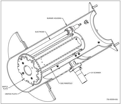
FIGURE 1-4. Burner Housing with a UV Scanner
