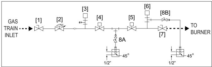
FIGURE 3-2. Gas Train Leak Test
