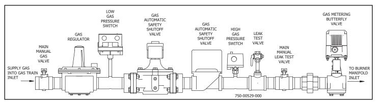
FIGURE 1-6. Main Gas Train for Full Modulation (Q6-055 to Q8-250)
