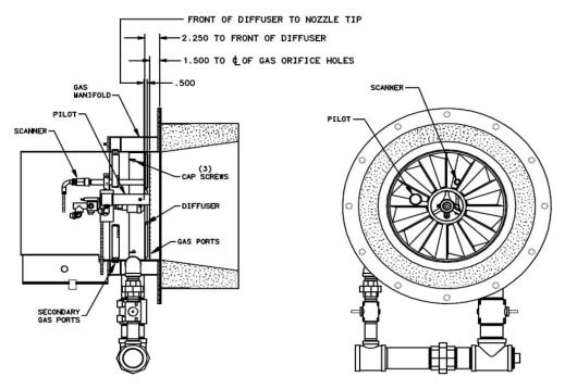
FIGURE 5-2. Firing Head Assembly: Dual Manifold
