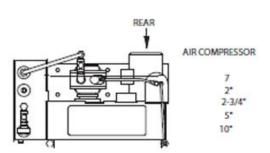
SEPARATE AIR COMPRESSOR MODULE **USED ON MODELS** DL, DLG, DM, DMG 175 TO 420 DE, DEG 42 TO 420
