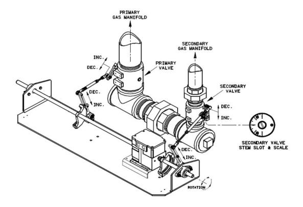
FIGURE 4-1. Gas Primary and Secondary Valve Arrangement: D 378-420
