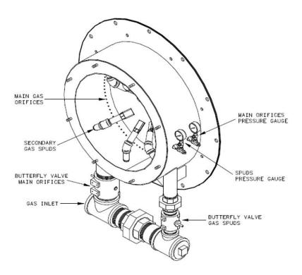
FIGURE 1-3. Dual Gas Manifold
