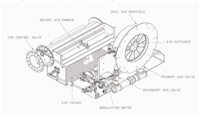
FIGURE 8-5. Secondary Gas Valve
