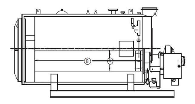
RECOMMENDED COMBUSTION CHAMBER DIMENSIONS - SCOTCH MARINE BOILERS
