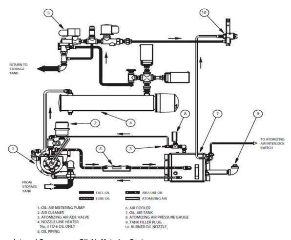
FIGURE 1-8. Integral Compressor Oil-Air Metering System
