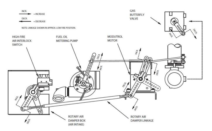
FIGURE 4-6. Firing Rate Control Adjustments
