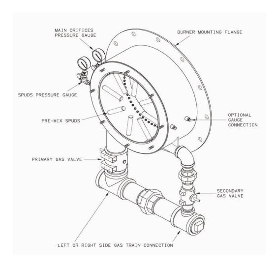
FIGURE 8-6. 20 PPM Head Assembly
