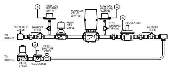
TYPICAL UL GAS PIPING OVER 5,000,000 UP TO 12,500,000 BTU - FULL MODULATION - MODELS D, LN 54 TO 105
