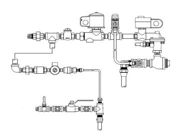
The nozzle line air purge option is used to purge the oil out of the nozzle line using the air compressor on a burner shutdown. The air purge line is mounted and piped on the burner. The air line from the compressor to the air purge line is by others.
