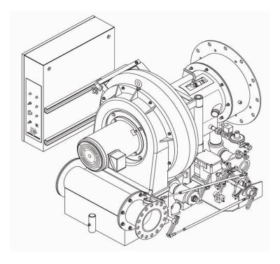
FIGURE 8-1. General Layout of the Burner
