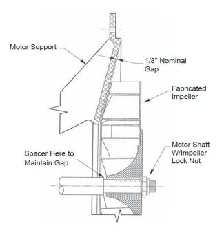
Proper clearance between the impeller and the inlet housing and between the impeller and stator cone is not critical and is set at 1/8" nominal. When installing or removing the impeller, it is mandatory to use an impact wrench.
