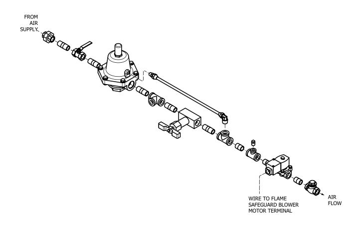
FIGURE 7-3. Plant Air System/Top Loaded with Air
