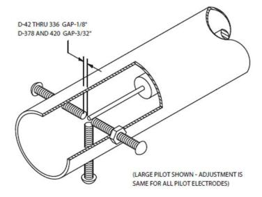
FIGURE 5-4. Ignition Pilot Electrode Setting
