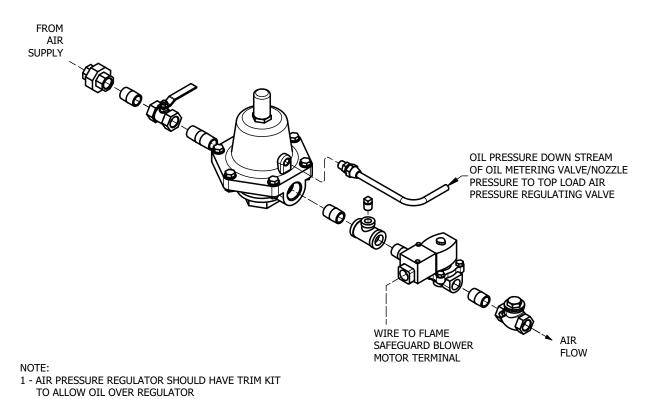
FIGURE 7-4. Plant Air System/Top Loaded with Oil
