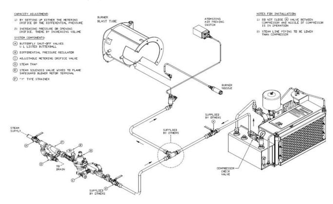
FIGURE 7-1. Steam Atomizing System
