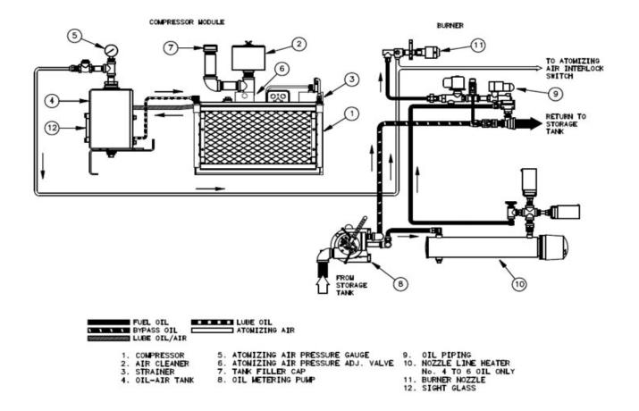
FIGURE 1-9. Compressor Module and Burner Oil Flow
