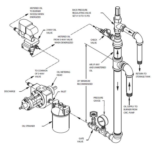
FIGURE 2-6. Typical Oil Supply Loop
