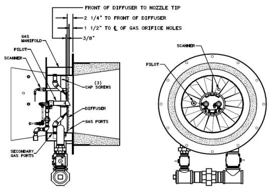
FIGURE 5-3. Firing Head Assembly: D378 & 420
