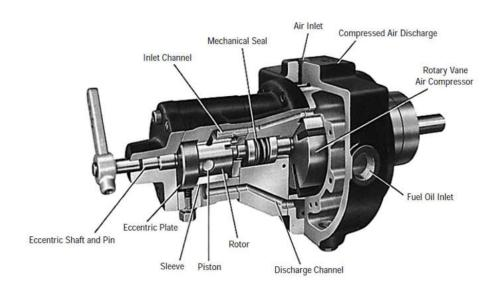
FIGURE 1-5. Integral Air/Oil Unit
