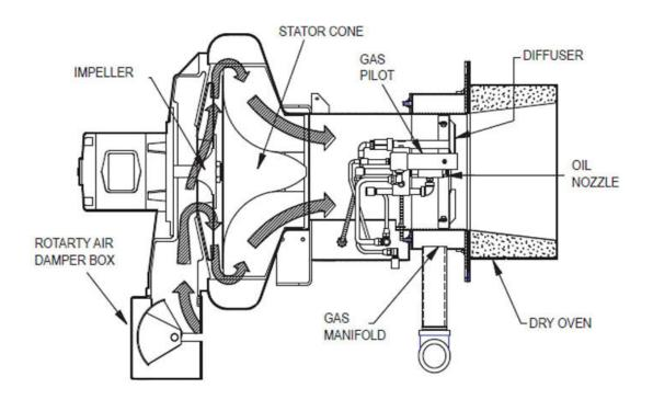
FIGURE 1-1. Damper, Impeller, and Stator Cone
