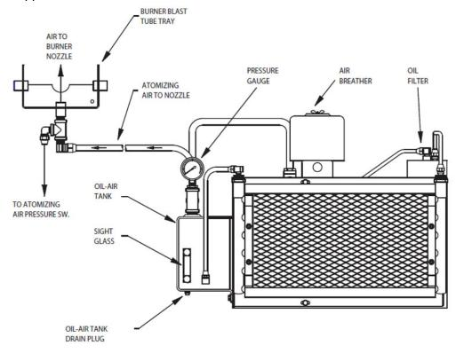
FIGURE 2-5. Separate Compressor Module
