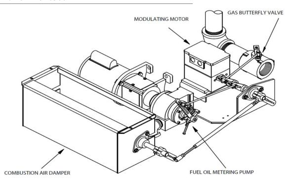
FIGURE 4-4. High Fire Position
