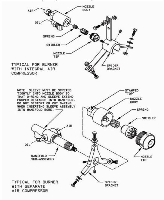
FIGURE 5-5. Oil Nozzle Assemblies
