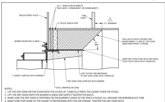
BURNER MOUNTING DETAILS FOR SCOTCH MARINE BOILERS
