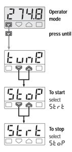
The green led comes on when Fuzzy Tuning is in progress. At the end of this operation, the calculated PID parameters are stored and used by the control algorithm, and the controller returns to the operator mode. The green led goes off.
