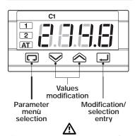
The parameter setting procedure has a timeout. If no keys are pressed for 30 seconds, the controller switches back, automatically, to the operator mode.
