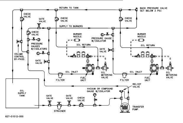
FIGURE 2-12. Typical Oil Loop for Multiple Burners with Transfer Pump
