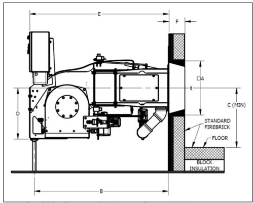
FIGURE 2-6. Standard Gas/Oil Configuration for Watertube/Cast Iron Boiler
