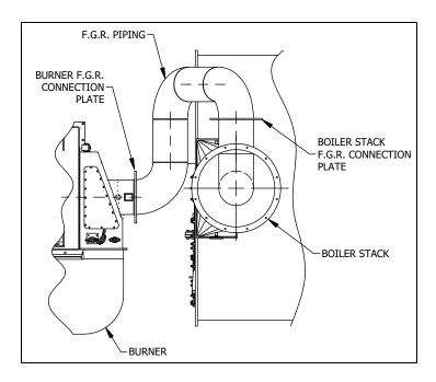
FIGURE 7-2. FGR Connection to Boiler - Top View
