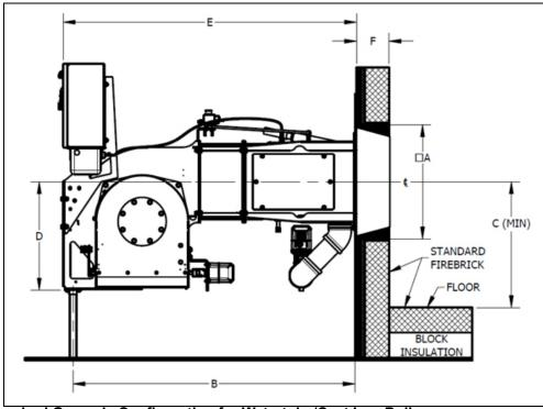
FIGURE 2-5. Standard Gas only Configuration for Watertube/Cast Iron Boiler
