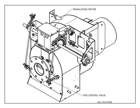
FIGURE 7-5. FGR Control Valve - High-Fire Position
