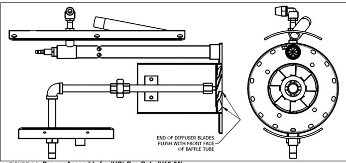
FIGURE 4-3. Drawer Assembly for (VG) Gas Only (V13-35)
