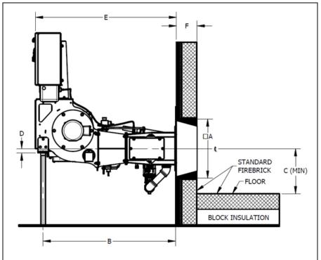
FIGURE 2-7. Inverted Gas Only Configuration for Watertube/Cast Iron Boiler
