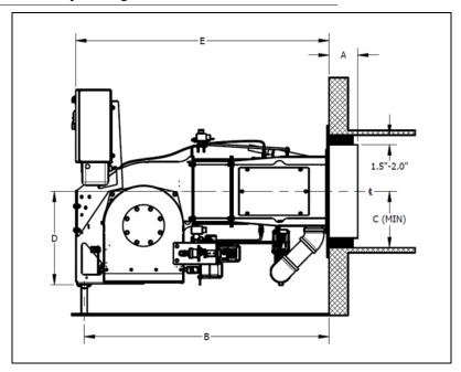
FIGURE 2-2. Standard Gas/Oil Configuration for Firetube Boiler
