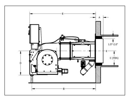
FIGURE 2-1. Standard Gas Only Configuration for Firetube Boiler
