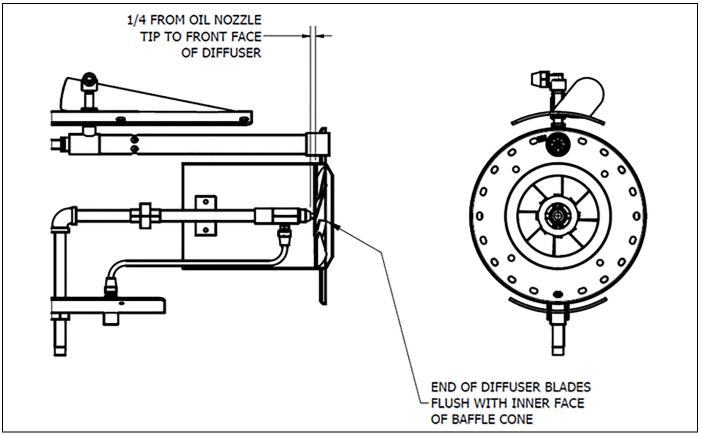
FIGURE 4-8. Drawer Assembly for (VLG) Gas/Oil (V40-55)
