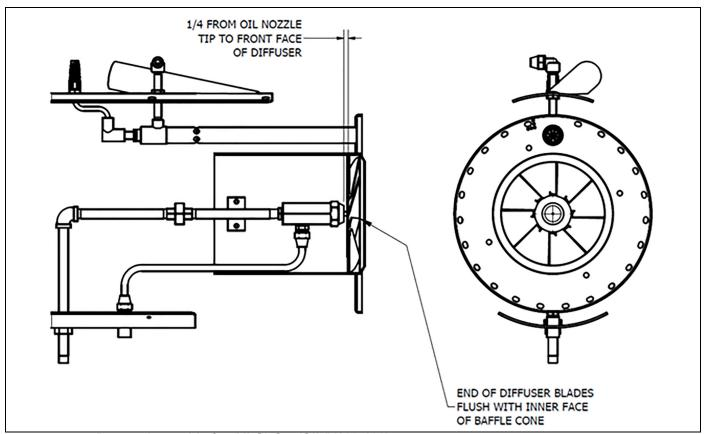
FIGURE 4-12. Drawer Assembly for (VLG) Gas/Oil (V120-168)
