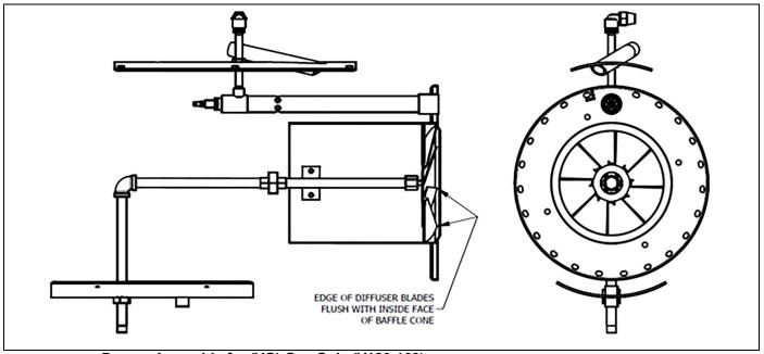
FIGURE 4-11. Drawer Assembly for (VG) Gas Only (V120-168)
