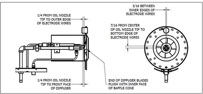
FIGURE 4-7. Drawer Assembly for (VL) Oil Only (V40-55)
