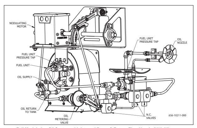
FIGURE 1-6. Full Modulation Oil System with Integral Pump & Return Flow Nozzle (V13-55)
