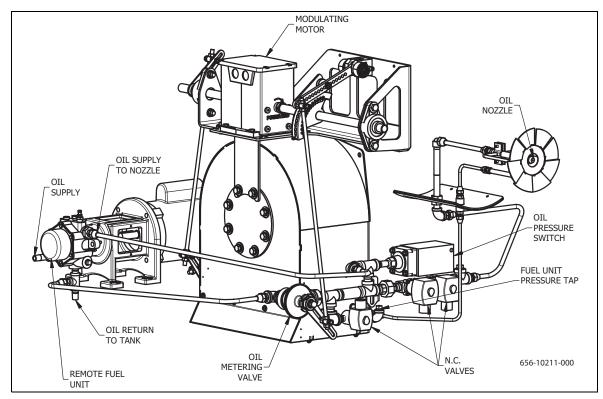
FIGURE 1-7. Full Modulation Oil System with a Remote Pump (V60-168)
