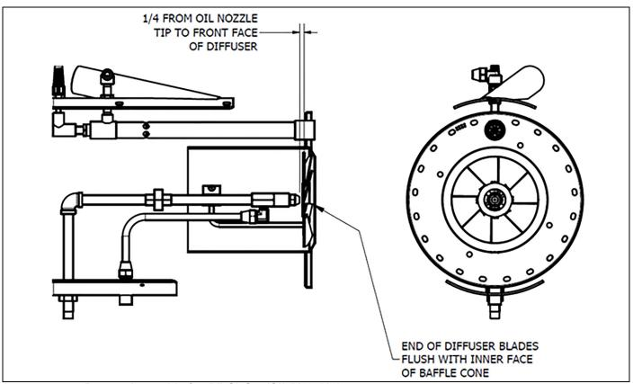
FIGURE 4-10. Drawer Assembly for (VLG) Gas/Oil (V60-110)
