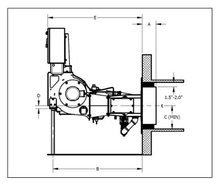
FIGURE 2-3. Inverted Gas Only Configuration for Firetube Boiler
