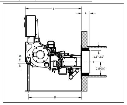
FIGURE 2-4. Inverted Gas/Oil Configuration for Firetube Boiler
