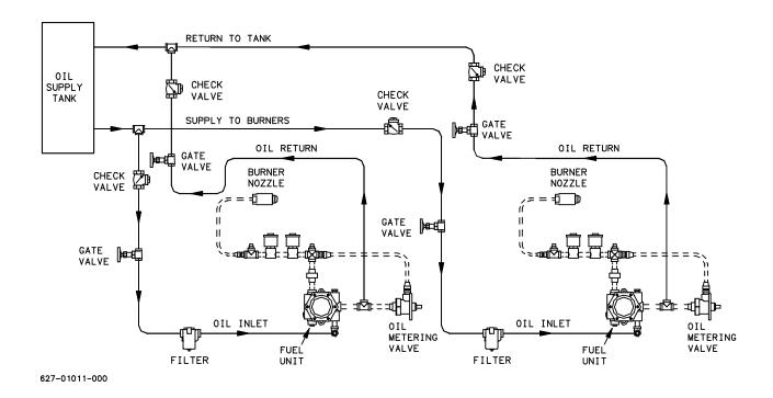
FIGURE 2-11. Multiple Burners with Separate Suction Lines
