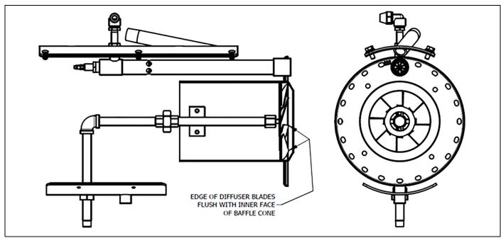
FIGURE 4-6. Drawer Assembly for (VG) Gas Only (V40-55)
