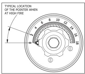
FIGURE 4-13. Oil Metering Adjustment Knob
