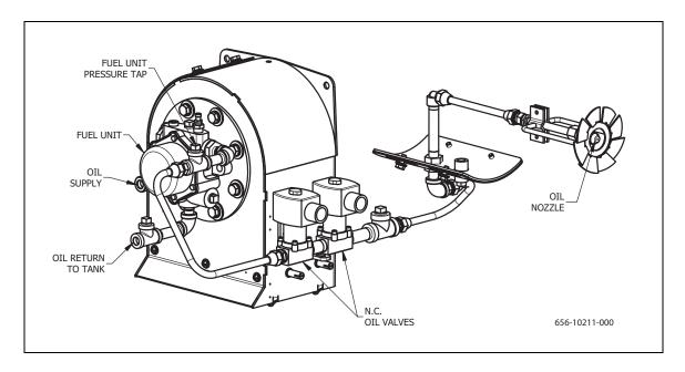
FIGURE 1-2. On-Off Oil System with Integral Pump & Simplex Nozzle (V13-25)
