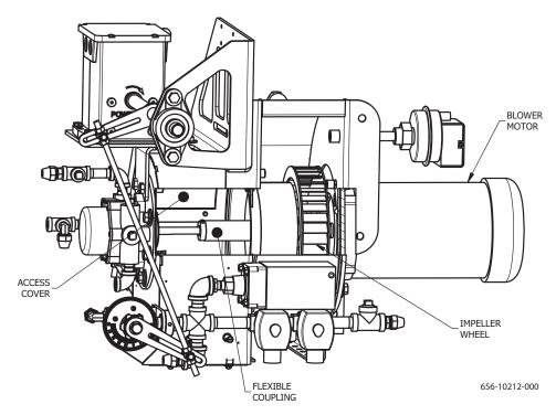
FIGURE 5-1. Air Handling System
