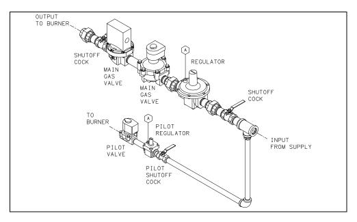
FIGURE 1-8. Typical Gas Train for On-Off System (V13-25)
