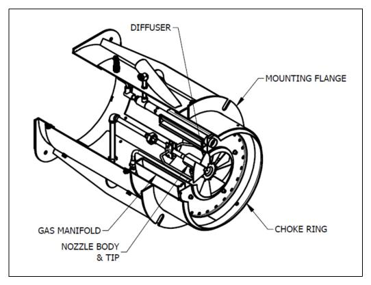
FIGURE 1-1. Burner Housing
