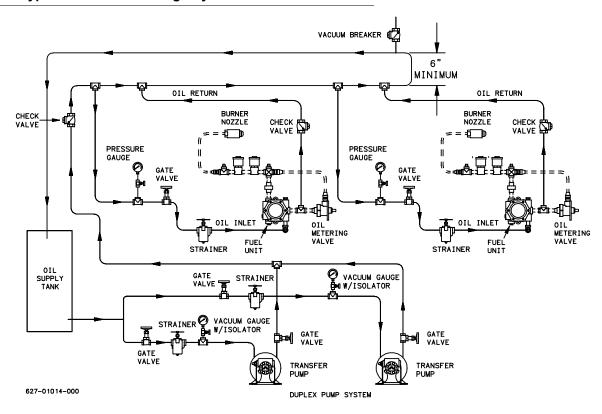
FIGURE 2-14. Typical Flooded Loop System
