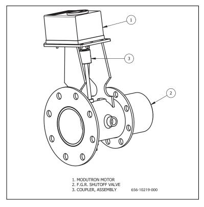
FIGURE 7-3. FGR Shutoff Valve
