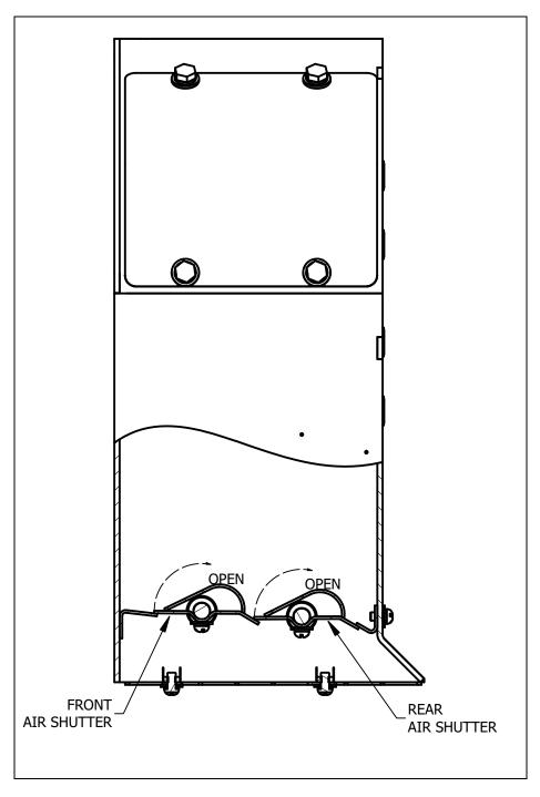
FIGURE 4-16. Front and Rear Shutters
