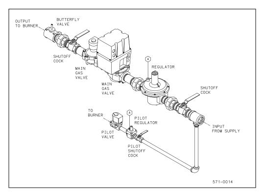
FIGURE 1-10. Typical Gas Train for Full Modulation System (V13-34)
