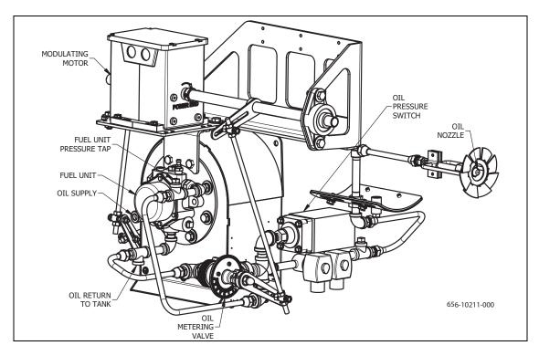
FIGURE 1-5. Full Modulation Oil System with Integral Pump & Simplex Nozzle (V13-34)
