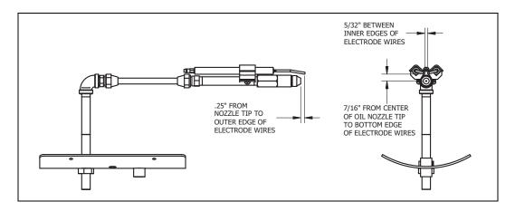
FIGURE 4-1. Direct Spark Ignition - Oil Only (VL) (V13-55)
