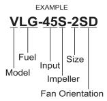
**Example:** The model number on the nameplate is **VLG-45S-2SD**. This is a No. 2 oil and gas burner with input rated at 4,500 MBtu/hr, it has a standard impeller, it is a Size 2 burner, and fan housing orientation is scroll down.
