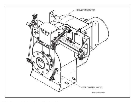
FIGURE 7-4. FGR Control Valve - Low-Fire Position
