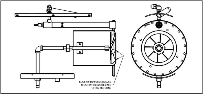
FIGURE 4-9. Drawer Assembly for (VG) Gas Only (V60-110)
