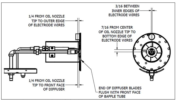
FIGURE 4-4. Drawer Assembly for (VL) Oil Only (V13-35)
