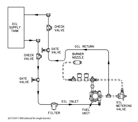
FIGURE 2-10. Typical No. 2 Oil Loop Single Burner
