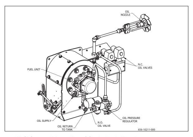
FIGURE 1-3. LHL Oil System with Integral Pump & Simplex Nozzle (V13-34)
