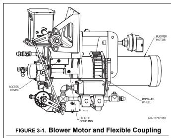
**NOTE:** Size 1 & 2 combination gas/oil units use a direct coupling from the blower motor to the oil pump. When firing gas for an extended period of time, the coupling should be manually removed and replaced only when firing oil. If the coupling is left connected to the blower motor, ensure that there is proper oil circulation at all times to avoid damage to and seizure of the pump.
