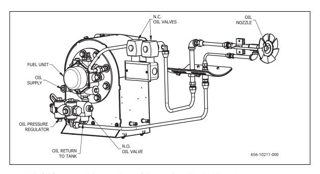
FIGURE 1-4. LHL Oil System with Integral Pump & Return Flow Nozzle (V13-55)
