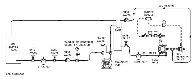
FIGURE 2-13. Typical Installation Using Day Tank
