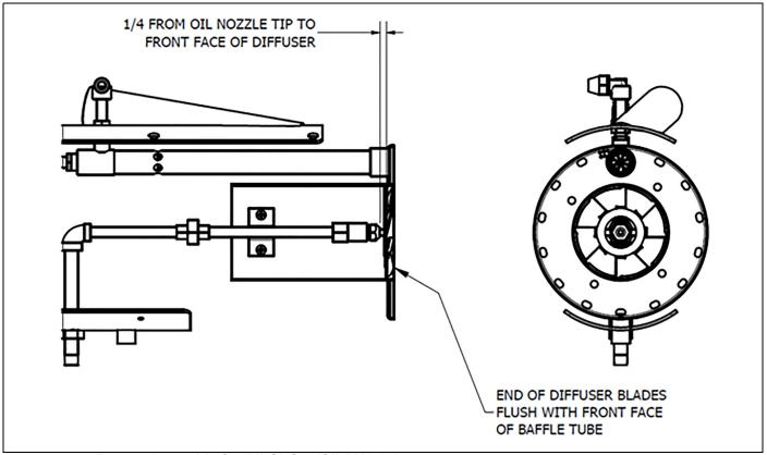
FIGURE 4-5. Drawer Assembly for (VLG) Gas/Oil (V13-35)
