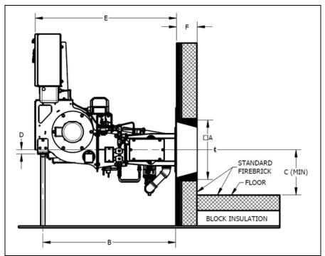
FIGURE 2-8. Inverted Gas/Oil Configuration for Watertube/Cast Iron Boiler
