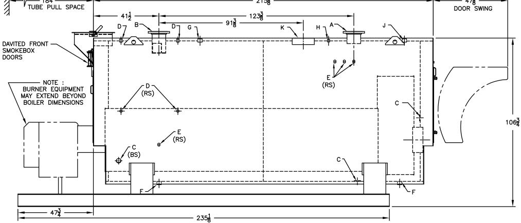
SPECIFICATIONS SUBJECT TO CHANGE WITHOUT NOTICE ALL CONNECTIONS ARE THREADED UNLESS OTHERWISE SPECIFIED MODEL 4SPW-400 431.5 BHP 125 PSI WATER
